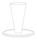
When attaching the marble top, please ensure that the metal conical base is placed in a fully vertical position prior to attaching.
